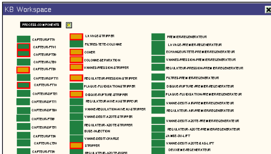
Figure 11: Visualisation of faulty and non-faulty components
